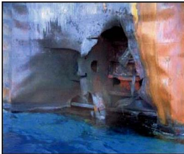
Figure 6.2.3-2: Close-Up of Hole in Hull of Limburg
